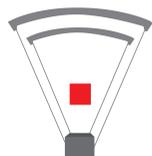
SuperChrono detection area superimposed on an ISSF 300m target.
