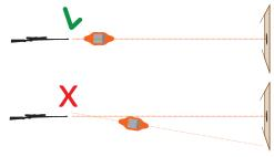
3. Find the height from the chronograph up to the line between the muzzle and the point of impact on the target, for example 30 cm. Using the sights, aim the chronograph 30 cm below the point of impact.
