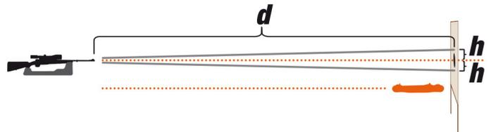
The distance  $h$  up or down from a true parallel bullet impact determines your precision. We use the same table as the one above. For a bullet speed of 2400 ft/s and target distance 100 yards, you can shoot 10 inches above or below the line from muzzle and target to get 99% precision or better.
