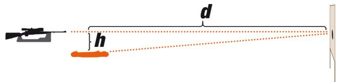
The letter  $d$  is used for distance and  $h$  for height;  $d$  is measured from the SuperChrono to the target and  $h$  is the distance between the SuperChrono's sensors and the line from the muzzle to the target.
