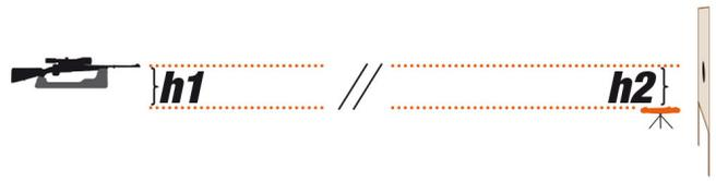
In this case you have to take care in aligning the sensors parallel with the line from the muzzle to the target.
